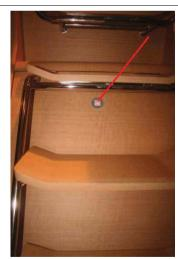
Extinguisher hole located under the companionway step (Reference 2)
