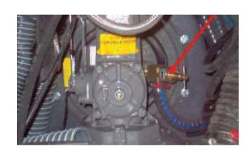
Engine water valve: On the sail-drive (Reference 2)
