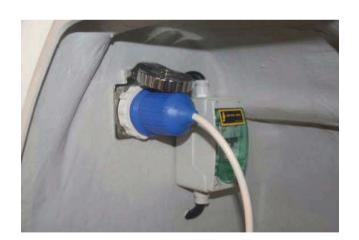
Access to platform socket and to bipolar switch from the port cockpit box in aft bulkhead
